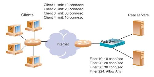
Figure 7-5 Configuring Clients with Different Rates
